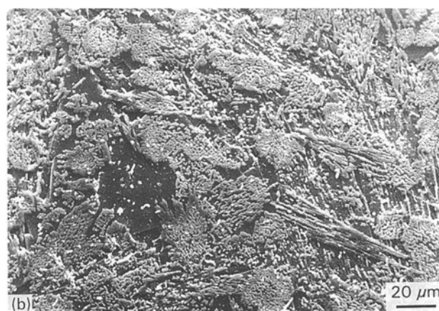
Figure 4 SEM photomicrographs of as-quenched glasses: (a) after a DTA run up to 1200^\circ\text{C} , (b) heated 4 h at 1200^\circ\text{C} .
